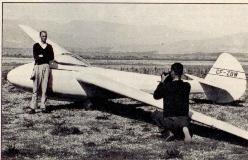
This is the same aircraft shown above. It has been modified with a bubble canopy, cleaned-up nose and wing roots and a takeoff dolly instead of the landing wheel.
