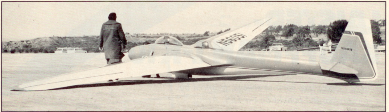
This L-K was modified greatly with separate bubbles for each cockpit, an extended rear fuselage, an enlarged vertical tail and a retractable main wheel.
