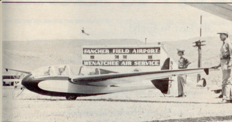
Simplest of all the clean-up modifications on the Laister-Kauffman was the bunny nose, which replaced the military's stepped windshield with extended molded plexiglass.
